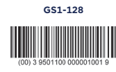
Item, box, case level GTIN with extended data or serial shipping container code (SSCC)
